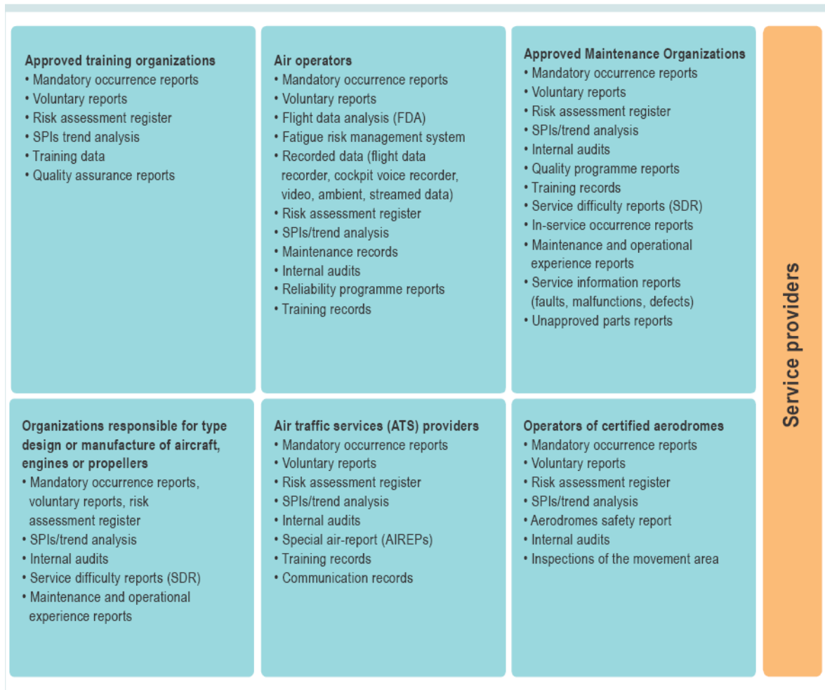
Figure 8-1 : Typical safety data and safety information sources
